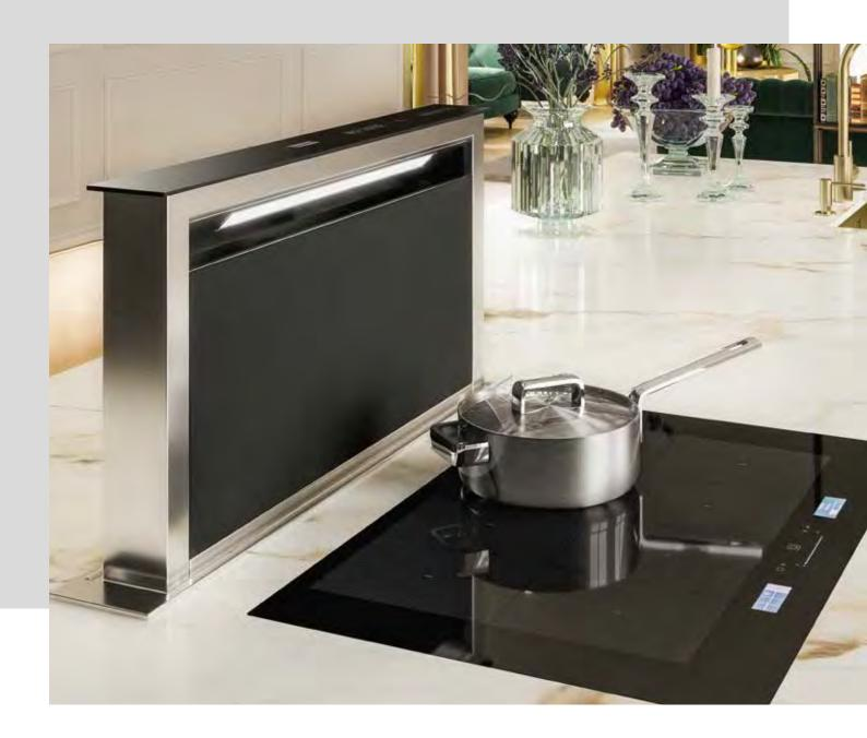
The motorised Downdraft hood allows for an unobtrusive, subtle kitchen style. The motor is situated in the cabinet underneath the hob which can be vented externally, or in recirculating mode. The motor can be installed at the front or rear according to the position of the kitchen unit. Compatible with gas, electric and induction hobs.
